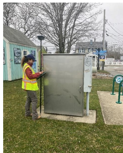
Figure 11: Critical Elevation Methods – High-Resolution LiDAR (Left) and In-Field RTK Surveying (Right)
